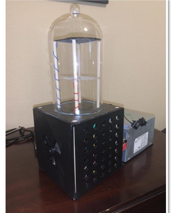
Self made radiation detector (cloud chamber)
