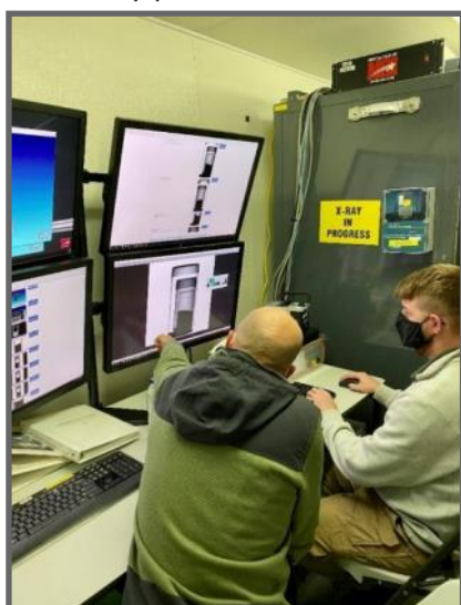
MPF team members assess X-ray images of cans of simulated plutonium.
