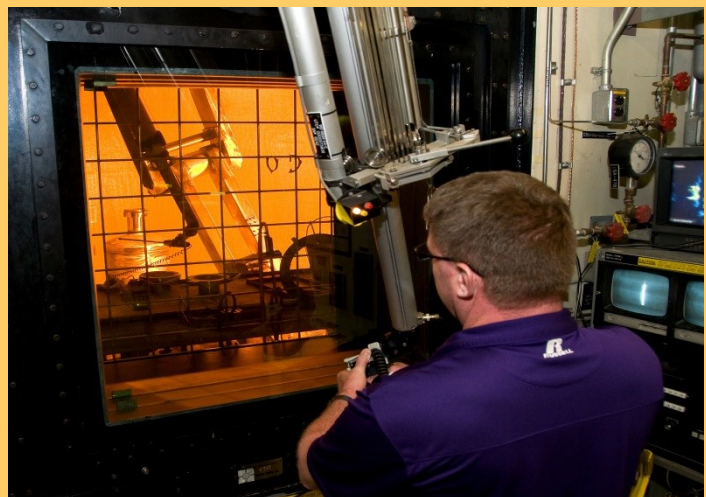
A Savannah River Remediation employee uses a manipulator arm during the filling of a canister inside the Defense Waste Processing Facility.
