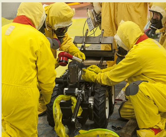
Operators modify a one-of-a-kind robotic recovery crawler used in H Canyon .
