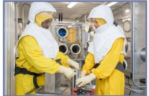
Savannah River Site radiation protection employees don protective equipment while working in a glovebox. Gloveboxes are structures with ports containing gloves that allow waste handlers to safely work with radioactive material.
