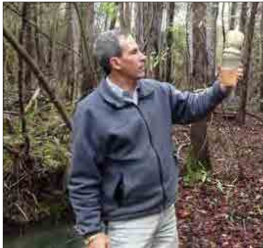
Visual assessment of an industrial stormwater outfall sample
