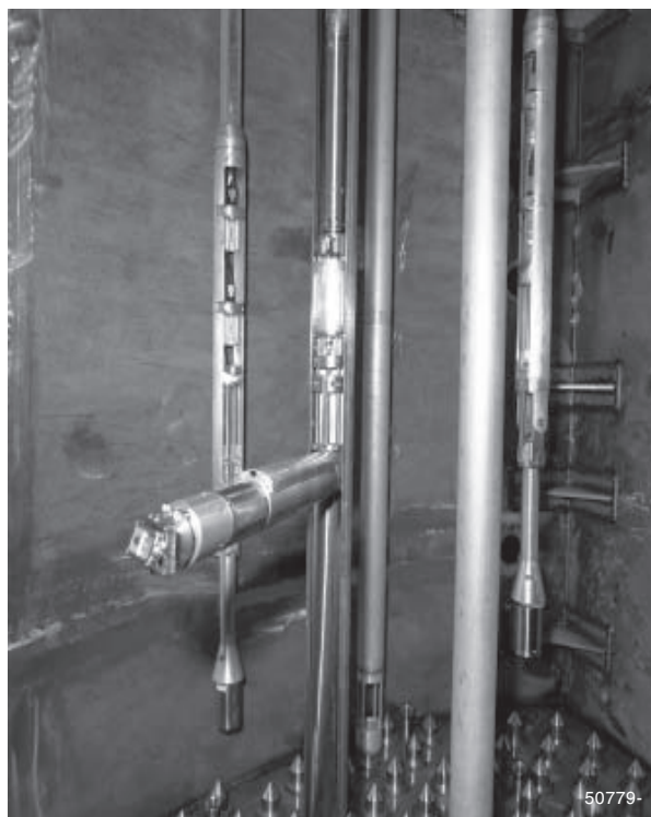
Figure 3. Reactor Tank Inspection Robot used to inspect welds in reactor vessels in
